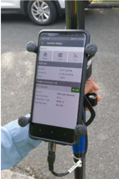
Plate 2.7 Trimble catalyst / DA1 GPS Antenna tested in the field – 29/9/19
