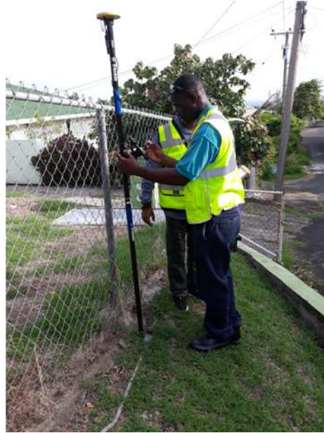
Plate 2.7 Trimble catalyst / DA1 GPS Antenna tested in the field – 29/9/19
