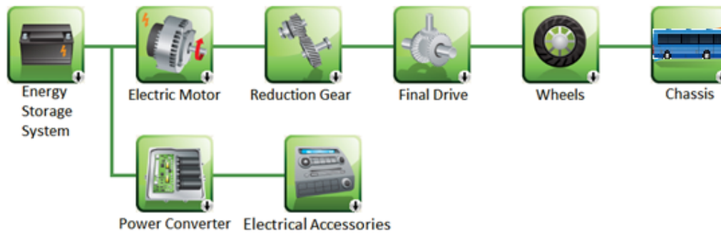
Figure 3. AUTONOMIE computational model of an electric bus powertrain. Each block is adapted to fit the specifications of the K7 electric bus.
