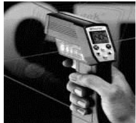
Figure 3.15: Infra Red Testing
