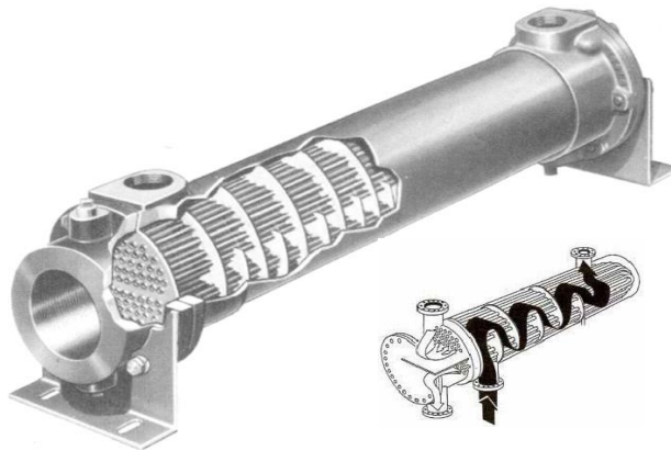
Figure 8.10: Shell-tube heat exchanger with one pass
