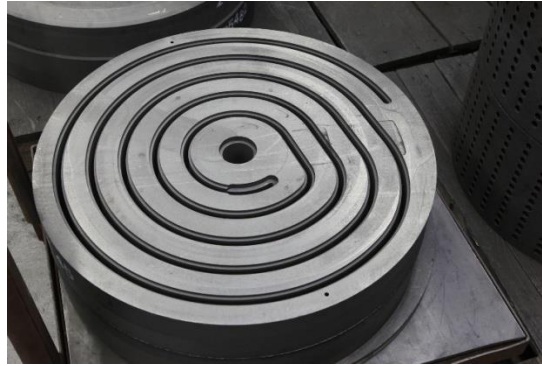
Source : GAB Neumann's Annular Grove graphite heat exchangers
