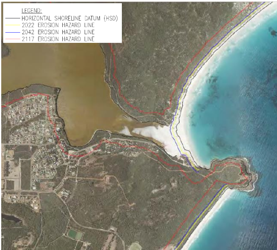
Figure 6.2. Coastal hazard lines for different temporal scenarios (Aurora Environmental, 2018).
