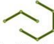
Simple multilinestring defined by 4 endpoints of 2 elements
