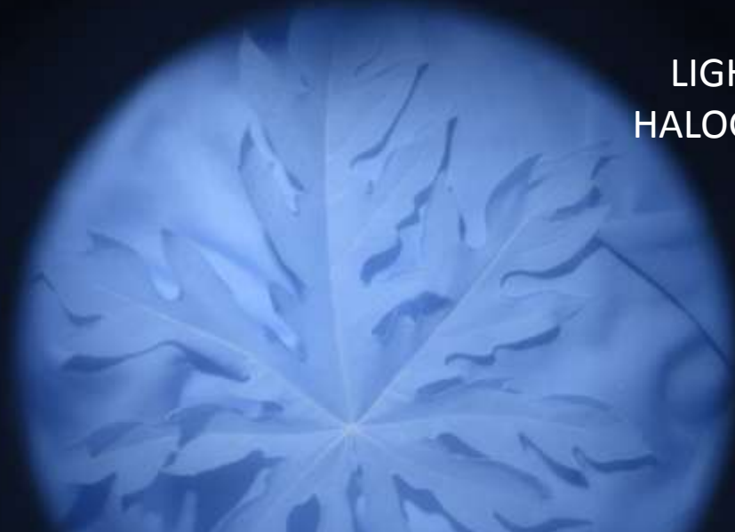
NIR CAMERA & PAPER FILTER (Longpass filter 590nm) ISO 200
