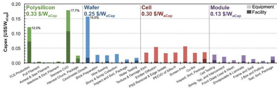
**Figure 4:** Costs of CapEx for manufacturing PV panels from Powell, et al., 2015.
