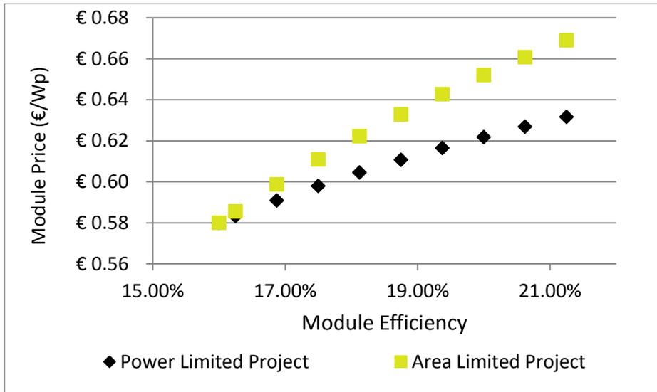
**Figure 2:** Potential value in Euro per kW depending on efficiency of solar panel
