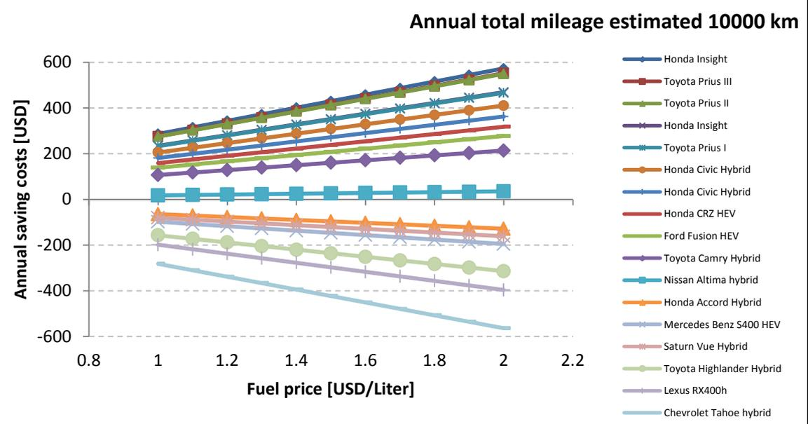
Figure 3. Annual operating saving costs of HEVs comparing to 2005 new fleet world average, as function of fuel price, with an annual mileage estimated 10000 km.
