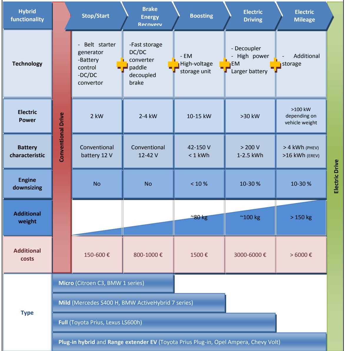
Figure 2. Power classification of existing electrified vehicles.
