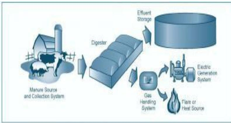
Figure 8: Main components of anaerobic digester facility
